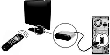
To use the remote control, point it in a direct line of sight at the remote sensor. The remote control and the sensor can be no farther than 8 meters (26 feet) apart. The remote control can be no more than 22.5 degrees (45 degrees total) from the center of the remote sensor.
