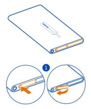
2 To unlock the SIM card holder, press and slide the holder to the left. Carefully pull out the holder.
