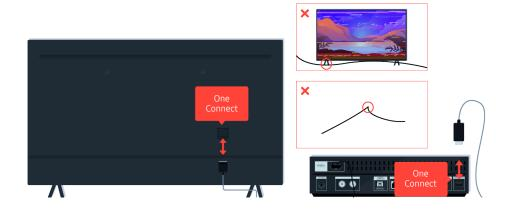
If the problem persists, and if your TV uses the One Connect, disconnect and reconnect the One Connect to the TV and the One Connect (OC) Box. Ensure that the One Connect is not pinched or bent sharply.
