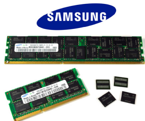
Figure 5. Samsung 40 nm Class, 1.35V High-Efficiency Green DDR3 Memory
