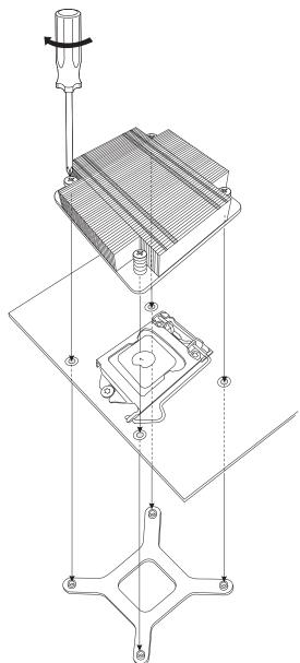
Figure 5-3. Installing the Heatsink
