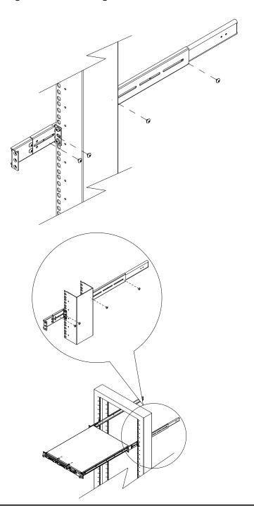
Figure 2-4. Installing the Server into a Telco Rack
