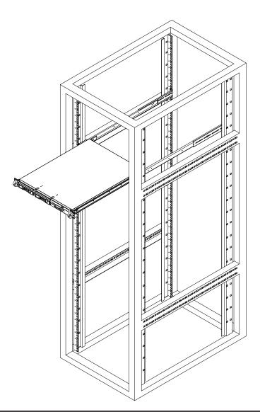
Figure 2-3. Installing the Server into a Rack
