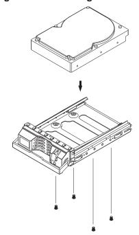
Figure 6-3. Mounting a Drive in a Carrier
