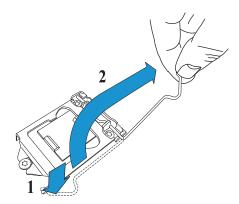
2. Gently lift the load lever to open the load plate. Remove the plate cap.
