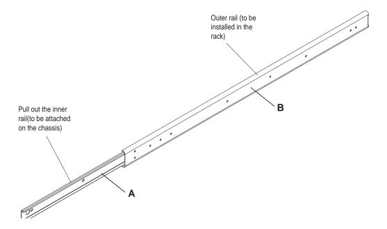
Figure 2-1. Identifying the Sections of the Rack Rails
