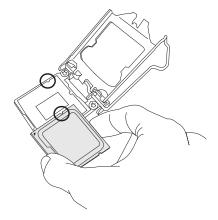
4. Align the CPU key that is the semi-circle cutouts against the socket keys. Once aligned, carefully lower the CPU straight down to the socket. (Do not drop the CPU on the socket. Do not move the CPU horizontally or vertically.
