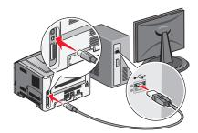
**Note:** After the printer is configured, the software will instruct you to disconnect the temporary USB cable so you can print wirelessly.
