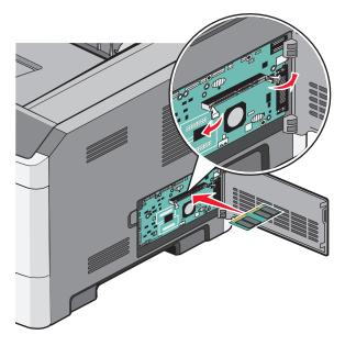
Additional printer setup 23 **4** Push the memory card into the connector until the latches *snap* into place.
