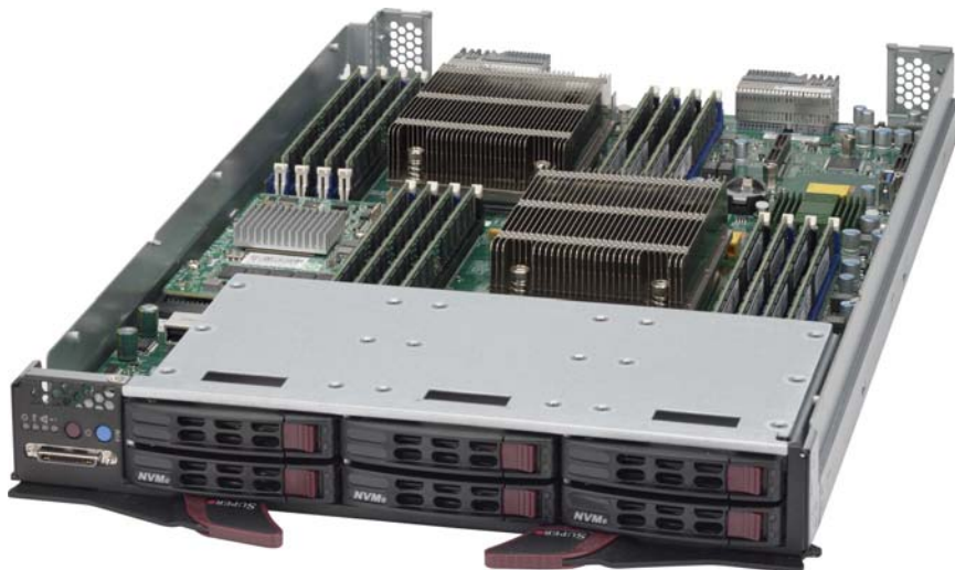
Figure 4-1. SBI-7128R-C6 Blade Unit Front View
