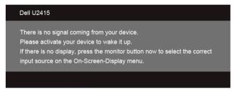
If either HDMI (MHL), Mini DisplayPort, or DP input is selected and the corresponding cable is not connected, a floating dialog box as shown below appears.
