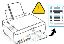
**EN** Scan the printed alignment page to complete setup. Go to step 4.
