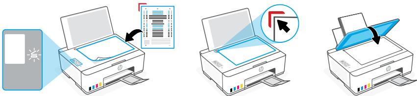
**EN** When the Open Lid light blinks, open the scanner lid and place the alignment page face-down on the scanner glass. Close the lid.
