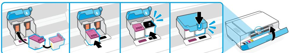
**EN** Position the electric contacts facing the printer, insert and click into place. Close the printhead cover properly, and then close the front door.
