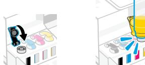
**EN** Open each tank cap and then fill all the tanks.
