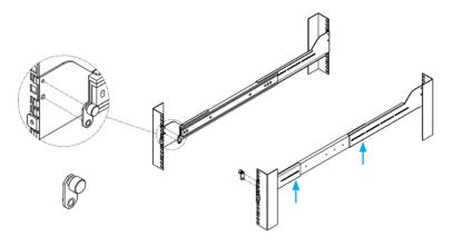
3. Slide the shelf assembly onto the rails.
