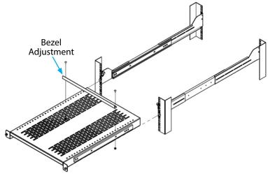
Attach the Cable Management Assembly to the back of the rack as shown.
