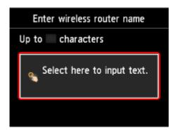
**4.** Enter the wireless router name (SSID). Text entry is case-sensitive.
