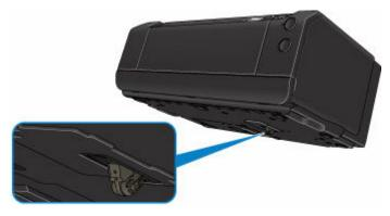
Place the printer as the ink supply stopper is properly grounded in hard flat surface such as a table.
