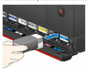
8. Firmly push the mark (PUSH) in front of the ink tank to secure it.
