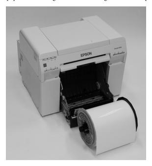
Load the roll paper spindle in the roll paper feeder with the gray adapter on the left. Check that the roll paper spindle fits between the rollers as shown.
