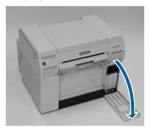
Be careful not to tilt the maintenance tank, and remove it carefully.
