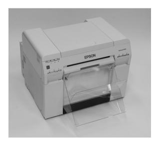
Tilt to insert the hooks, and then lower to hook it in place.
