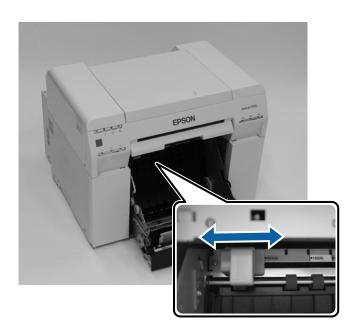
Hold the roll paper spindle in the orientation shown below, and place it in front of the roll paper feeder.
