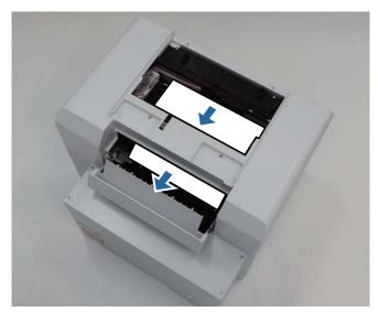
Move the print head manually, and remove the paper from the back of the printer.
