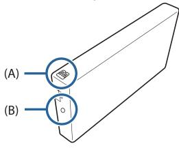
6 Slide the ink cartridge all the way into the printer.
