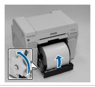
Push the roll paper feeder into the printer.
