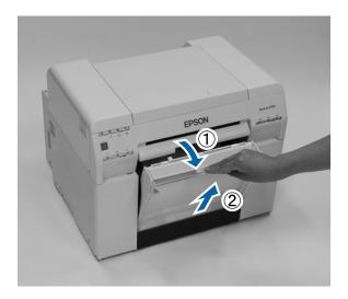
Grip the handle to release the roll paper feeder and then pull it out.
