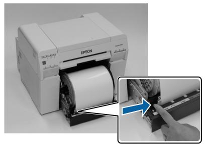
Insert the leading edge of the paper into the paper feed slot until the paper light turns on.
