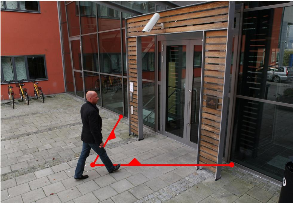
AXIS Cross Line Detection is a trip-wire application installable on Axis network cameras and encoders. The application detects moving objects that cross a virtual line making it possible to automatically trigger an event. AXIS Cross Line Detection will increase system efficiency by reducing bandwidth and storage needs and facilitate search of recorded events.
