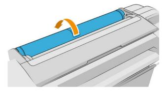
2. Remove the black end of the spindle from the printer, then the blue end.
