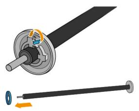
6. Slide the core onto the take-up reel. The core should be at least as wide as the paper.
