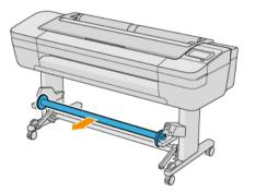
5. Lift the lever to unlock the paper stop from the take-up reel and put it aside.
