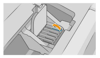
9. Using the blue handle, use steady force to disengage the printhead.
