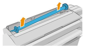
3. The spindle has a stop at each end to keep the roll in position. The blue stop can be removed to mount a new roll; it slides along the spindle to hold rolls of different widths. Remove the blue paper stop from the end of the spindle.
