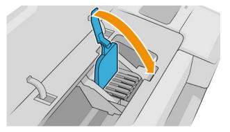
5. Ensure that the end of the blue handle catches the wire loop on the near side of the carriage.
