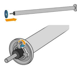
8. Load the take-up reel into the printer by pushing firmly on both ends.
