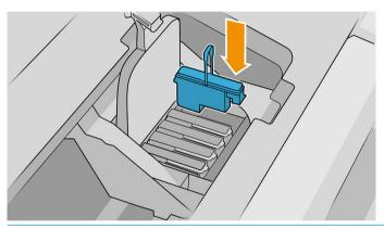
▲ CAUTION: When installing the new printhead there may be some resistance, so you need to press it down firmly but smoothly. You should hear a beep and see confirmation on the front-panel display that the printhead has been inserted. If you have difficulty, see <u>Cannot insert a printhead on page 170</u>.
