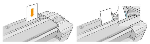
6. Load your sheet aligned with the load line and insert it until the paper will not continue; with thicker sheets, you feel resistance.
