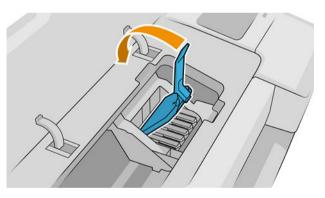
8. To remove a printhead, lift up the blue handle.
