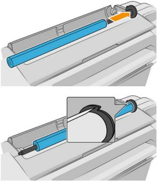
Ensure that the end of the roll is as close to the spindle stop as possible.
