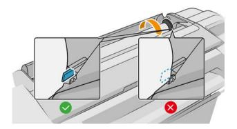
9. Roll the paper into the printer until you feel resistance and the paper flexes slightly. When the printer detects the paper, it beeps, then feeds it in automatically.
