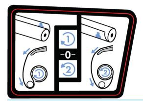
**14.** Tap the button on the front panel to advance the paper, creating a loop.
