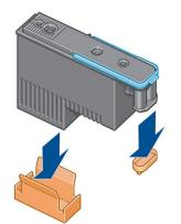
2. The printhead is designed to be inserted into any of the available slots. Once the printhead is inserted into a specific slot, it will be set up to work only with that combination of colors. For this reason, it is important to mark the printhead with its specific color, on the label that comes with it, matching the color of the carriage slot into which the printhead is to be inserted.
