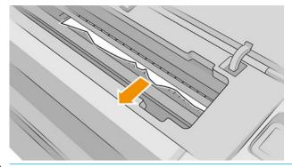
$\triangle$  CAUTION: Do not move the paper sideways, as it could damage the printer.
