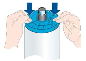
If you are a regular user of different paper types, you can change rolls more quickly if you preload rolls of different paper types on different spindles. Extra spindles are available for purchase, see <u>Accessories</u> on page 133.
