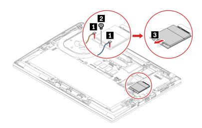
**Note:** During installation, ensure that you connect the cables with different colors to the corresponding connectors on the card according to the illustrations above: the orange cable to the connector labeled
