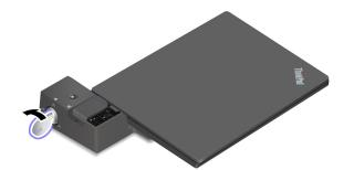
2. Slide the latch in the direction as shown **I** to release the computer, and then grasp both sides of the computer to remove it **I**.
