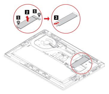
Removal procedure for the short M.2 solid-state drive and its bracket (for ThinkPad X13 Gen 2)
