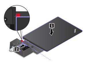
5. Check the docking status indicator. The docking status indicator turns on when the computer is successfully docked.
