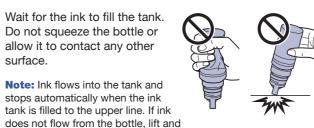
5 When the ink tank is full, remove the ink bottle and securely close it with the bottle cap. Place the remaining ink aside; you will need it later.
