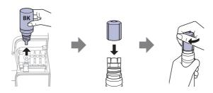
Note: Do not leave the ink bottle inserted; otherwise the bottle may be damaged or ink may leak. If any ink remains in the bottle, store the bottle upright and top off the ink tank after completing initial setup.
