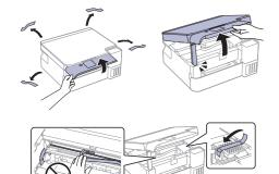
To close the scanner unit, lift the scanner unit slightly, then lower it until it stops. Repeat the motion to fully close the scanner unit.
