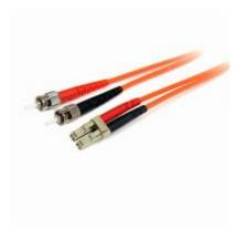
The FIBLCST5, 5-meter (16ft) Multimode 62.5/125 Duplex Fiber Patch Cable is terminated with one LC (male) connector and one ST (male) connector, to provide the necessary connection between fiber networking devices for high-speed, long distance networks.
