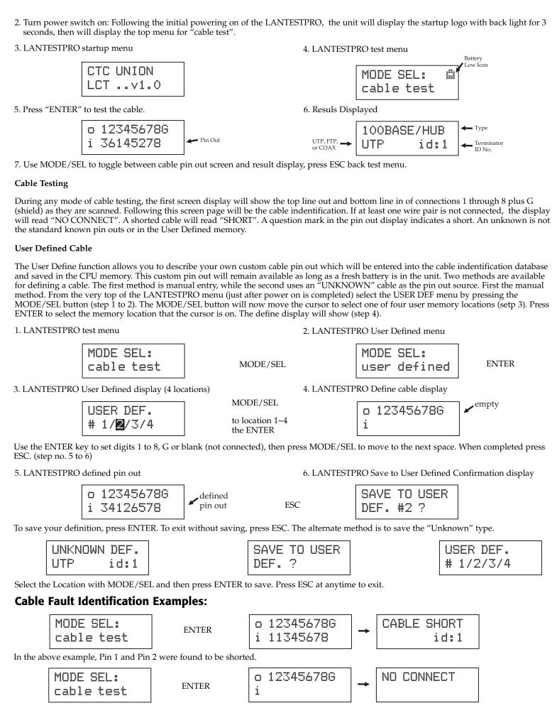
In the second example, if a least one pair of the wires is not connected, the test result will show as "NO CONNECT".
