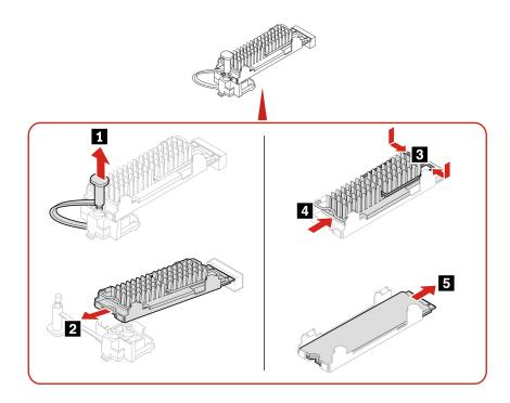
Note: When installing the M.2 solid-state drive and the heat sink, remove the film (if any) that covers the thermal pad.
