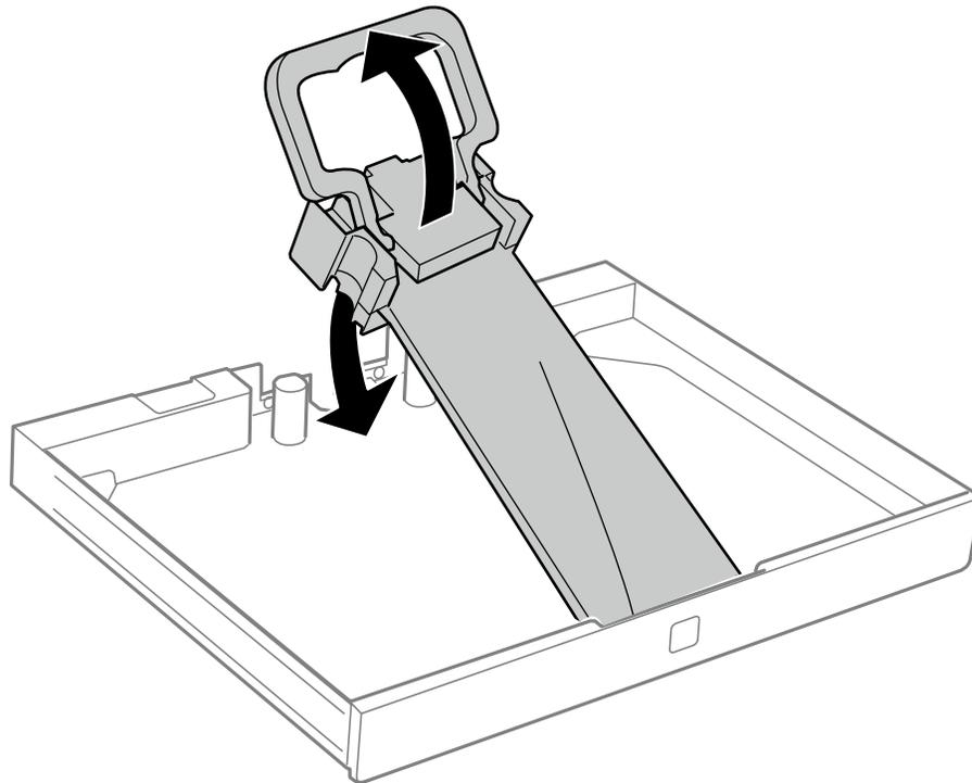
7. Make sure the top of the ink pack is level with the top of the tray and move the handle back to its original position.
