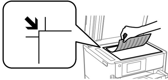
**Note:** The edges of your original may be cropped by 0.06 inch (1.5 mm) from the edge of the scanner glass. Manually position your original away from the edges to prevent cropping.
