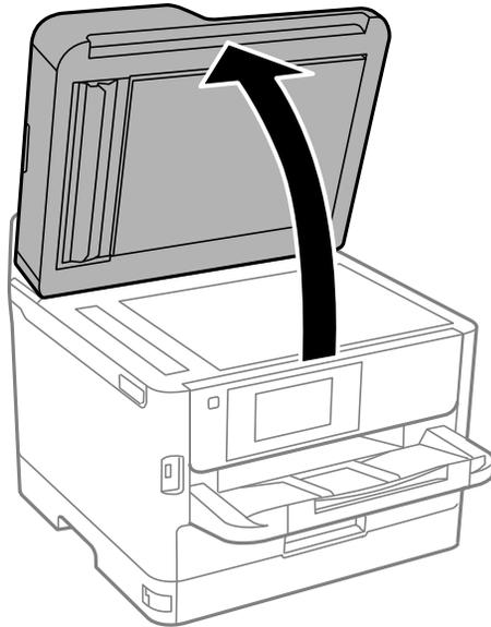
2. Place your original facedown on the scanner glass with the top facing into the corner. Slide the original to the edges of the indicated corner.
