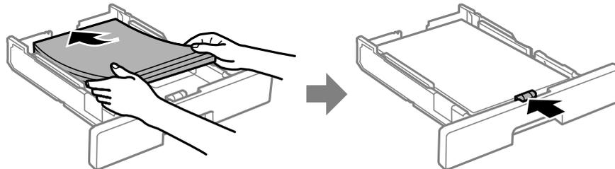
**Note:** Make sure the paper fits beneath the arrow mark inside the edge guides.
