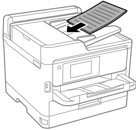
**Note:** Do not load originals above the arrow mark on the ADF edge guide.
