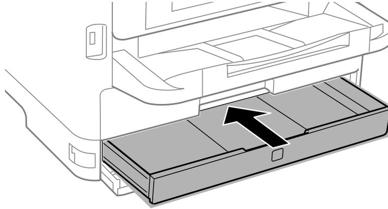
**Note:** If you cannot insert the tray all the way, make sure the top of the ink pack is level with the top of the tray.
