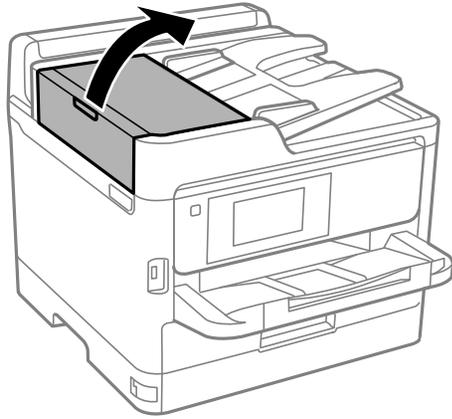
8. Use a soft, moist, lint-free cloth (microfiber is recommended) to clean the rollers and the interior of the ADF.
