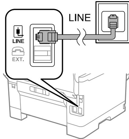
**Note:** If you have a DSL or ISDN connection, you must connect the appropriate DSL filter, or ISDN terminal adapter or router to the wall jack to be able to use the line for faxing or voice calls using your product. Contact your DSL or ISDN provider for the necessary equipment.
