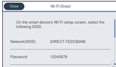
5. Use your computer or wireless device to select the Wi-Fi network name (SSID) displayed on the LCD screen, then enter the password shown.
