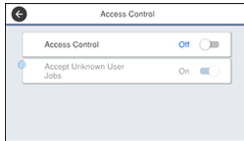
3. Select the **Access Control** field to turn the setting on.
