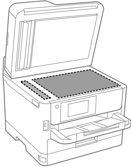
**Note:** If lines appear on the printout or in scanned images, carefully clean the scanner glass on the left.
