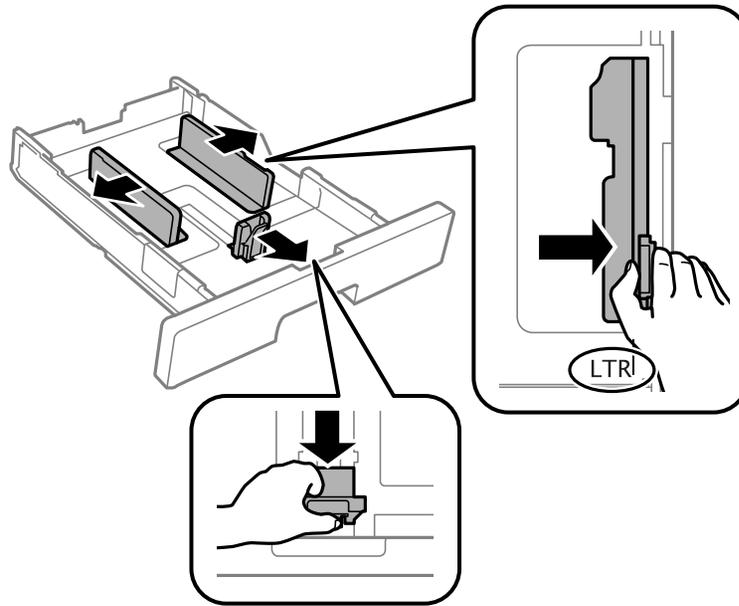
3. Load paper with the printable side facedown and slide the front edge guide against the paper.
