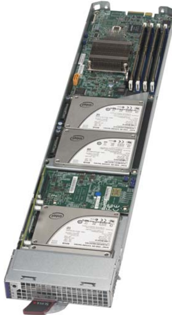
Figure 4-1. MBI-6118G-T41X Blade Unit Front View
