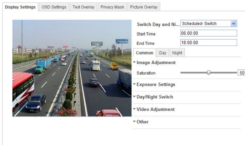
Figure 6-37 Day/Night Scheduled-Switch Configuration Interface
