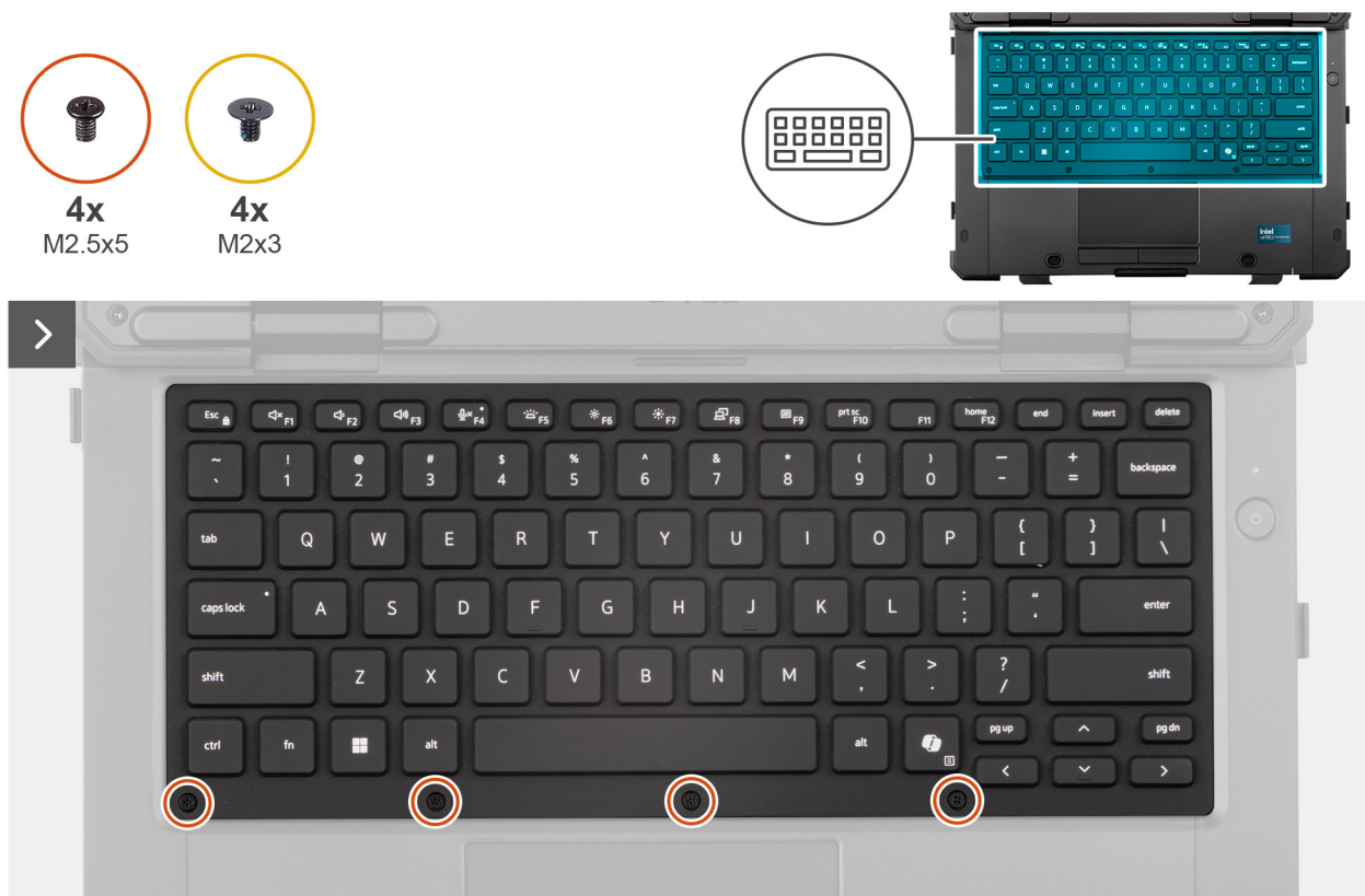
Figure 29. Removing the keyboard (rubberized)
