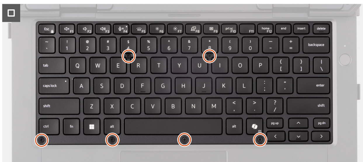
Figure 28. Installing the keyboard (standard)
