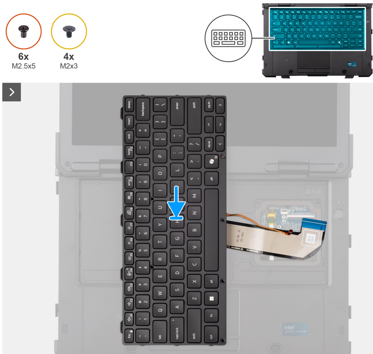
Figure 25. Installing the keyboard (standard)
