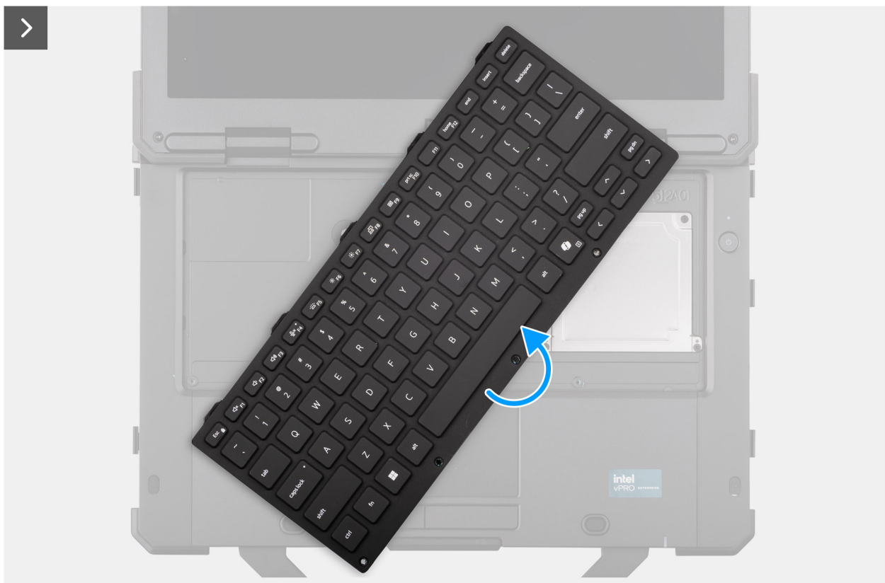
Figure 31. Removing the keyboard (rubberized)
