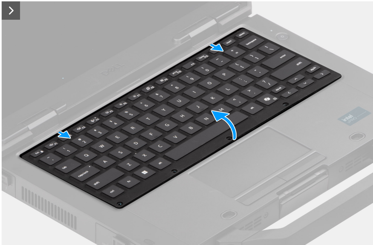
Figure 30. Removing the keyboard (rubberized)
