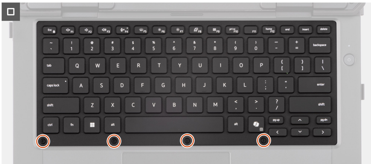
Figure 36. Installing the keyboard (rubberized)
