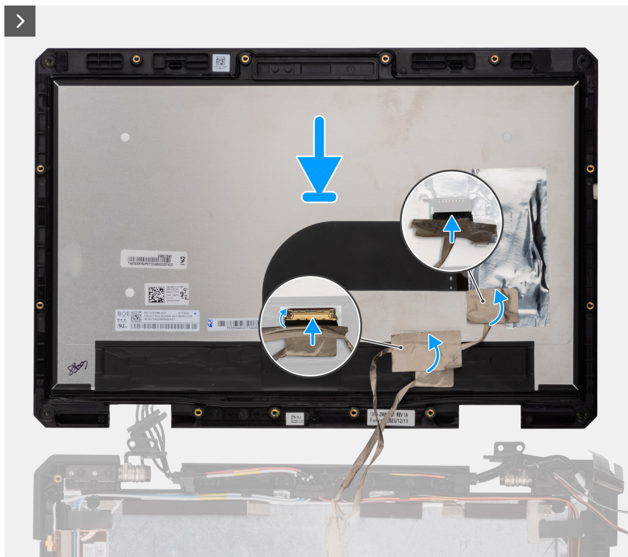
Figure 126. Installing the display-panel assembly
