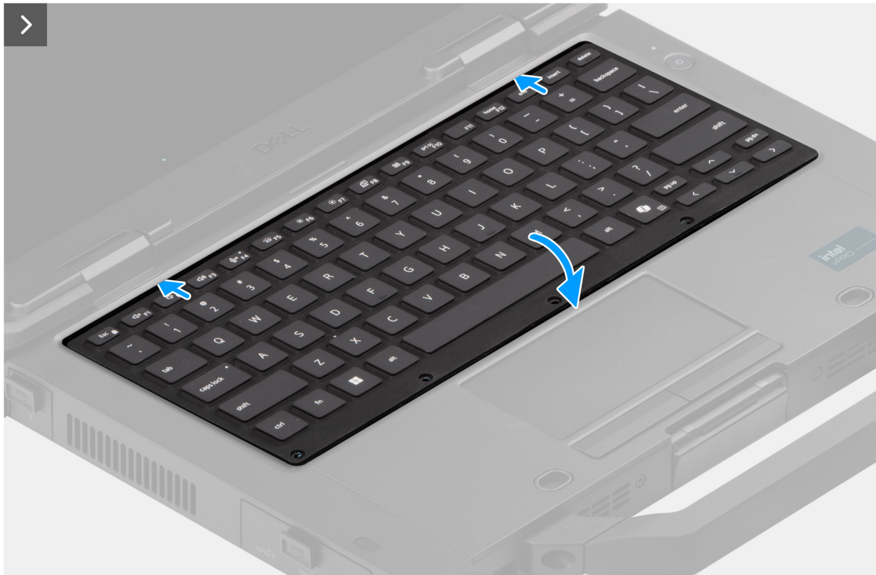
Figure 35. Installing the keyboard (rubberized)
