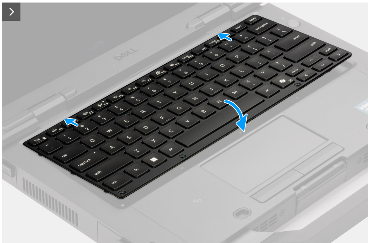
Figure 27. Installing the keyboard (standard)
