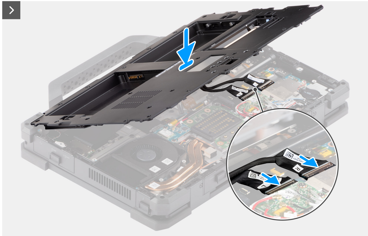
Figure 49. Installing the base cover
