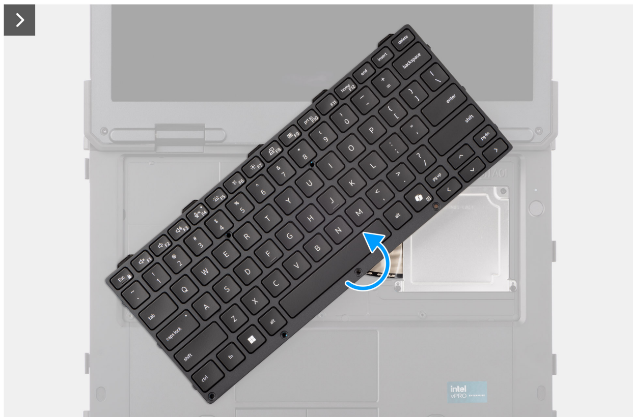
Figure 23. Removing the keyboard (standard)
