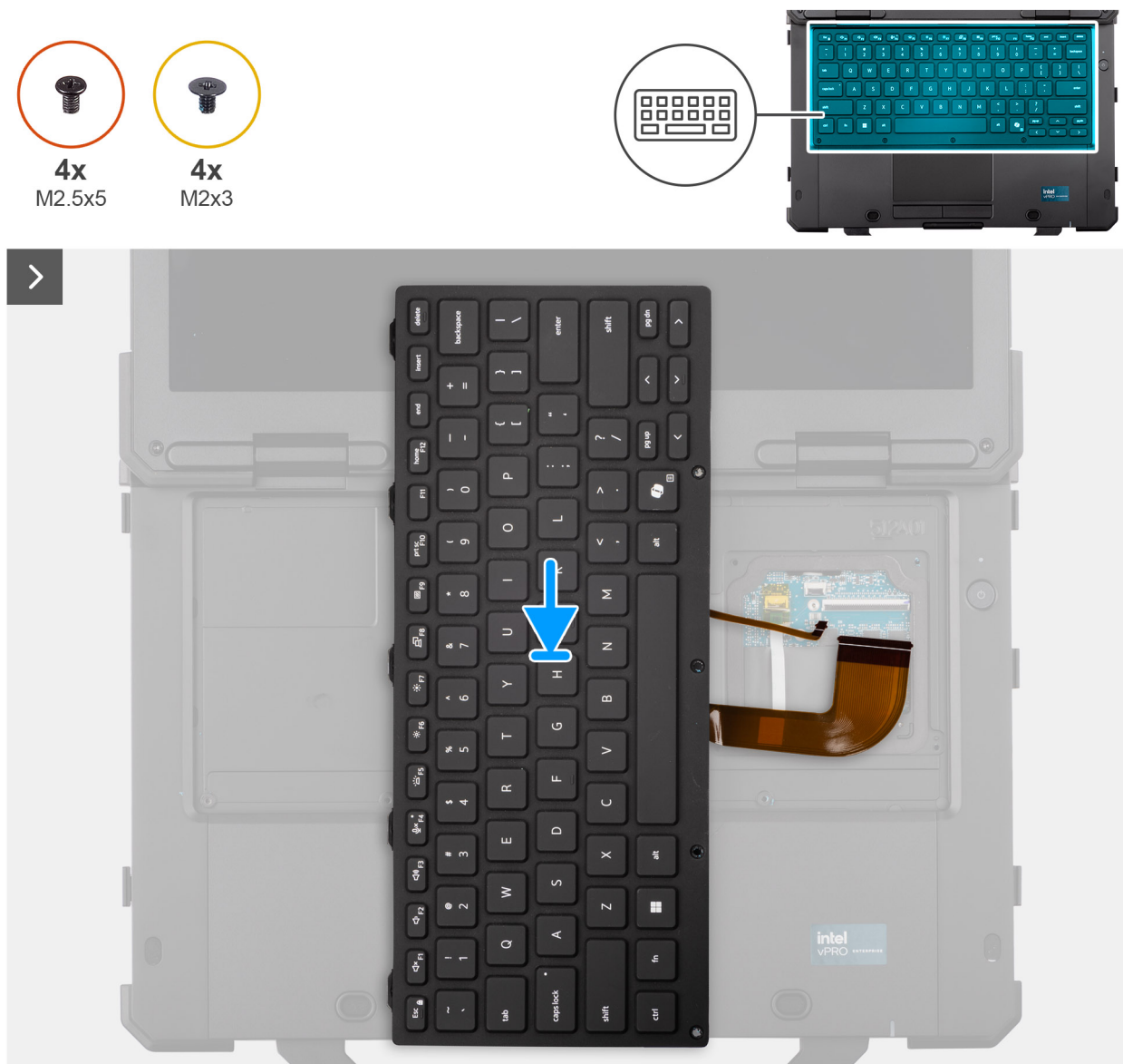
Figure 33. Installing the keyboard (rubberized)
