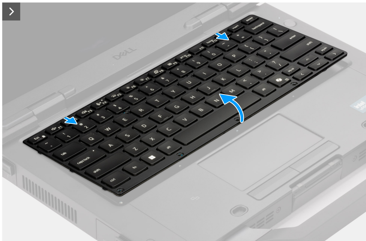
Figure 22. Removing the keyboard (standard)
