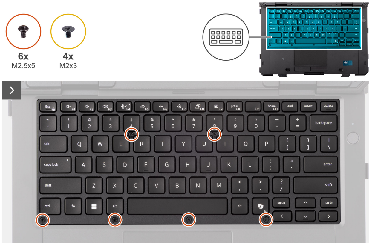
Figure 21. Removing the keyboard (standard)
