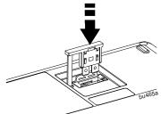
Slide the battery connector handle away from its Turn the battery connector to a 90-degree disconnected position.
