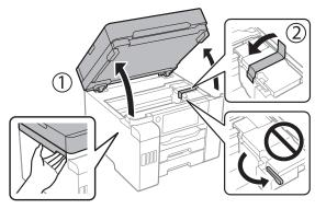
**Caution:** The printer ships with the transportation lock in the printing position. Do not move it from the printing position.
