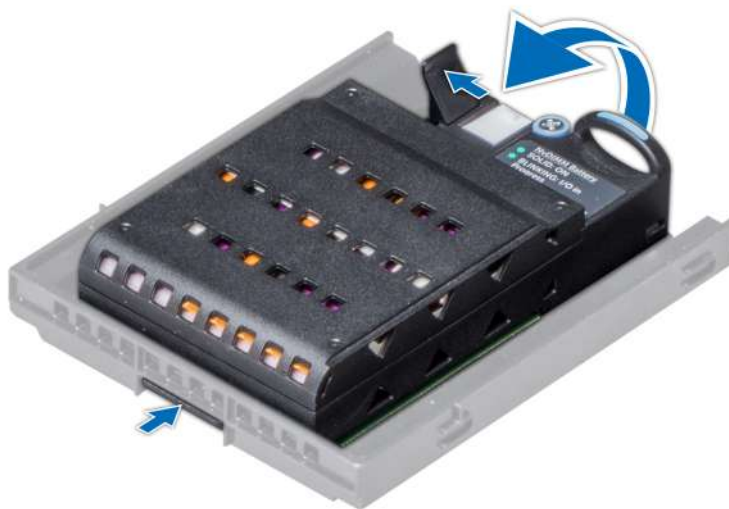
Figure 43. Removing NVDIMM-N battery from the bracket
