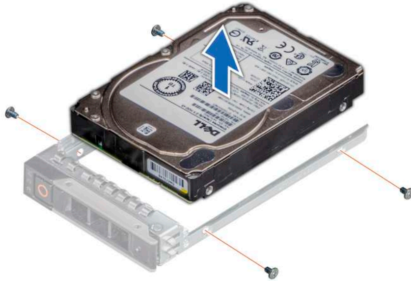
Figure 63. Removing the drive from the drive carrier
