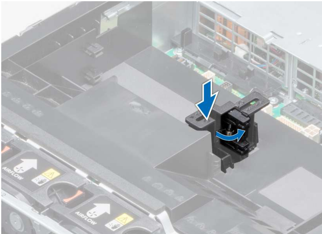
Figure 80. Opening the PCIe card holder latch
