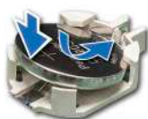
Figure 162. Installing the system battery
