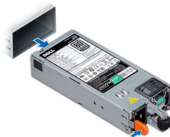
Figure 165. Removing a power supply unit
