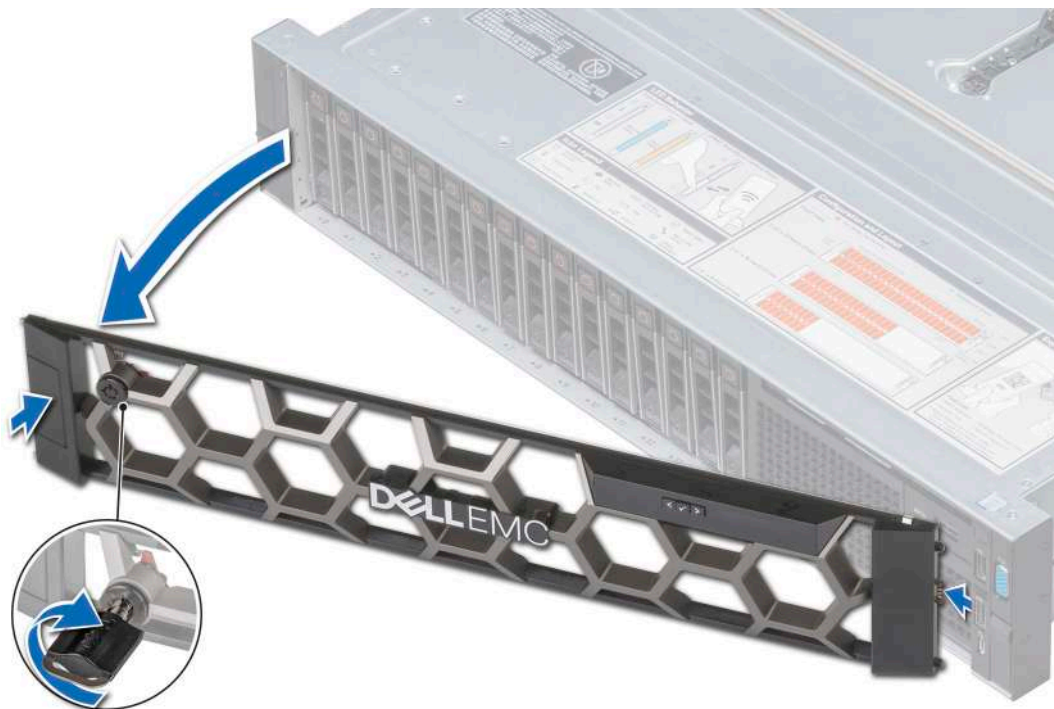
Figure 23. Removing the optional front bezel with the LCD panel
