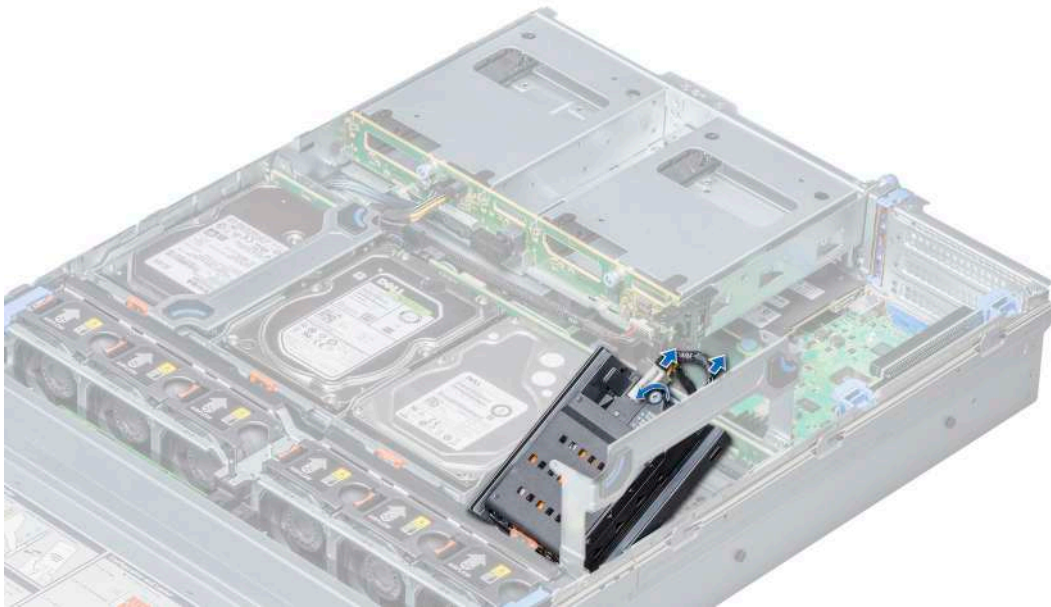
Figure 41. Removing NVDIMM-N battery from mid drive tray
