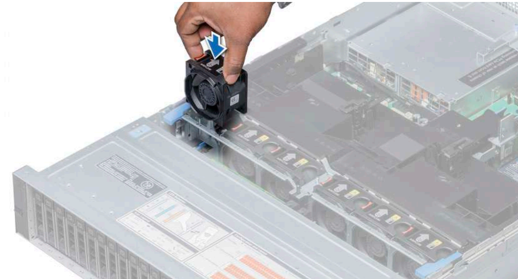
Figure 36. Installing cooling fan
