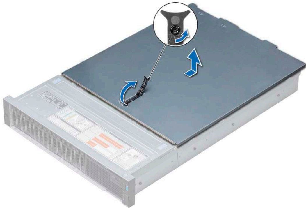
Figure 25. Removing the system cover
