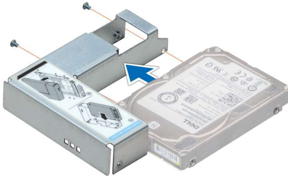
Figure 60. Installing a 2.5 inch drive into the 3.5 inch drive adapter
