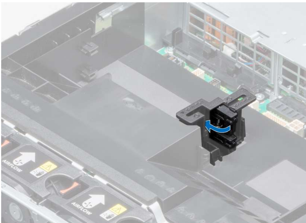
Figure 81. Closing the PCIe card holder latch
