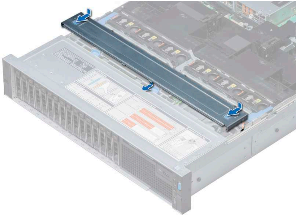
Figure 28. Installing the backplane cover
