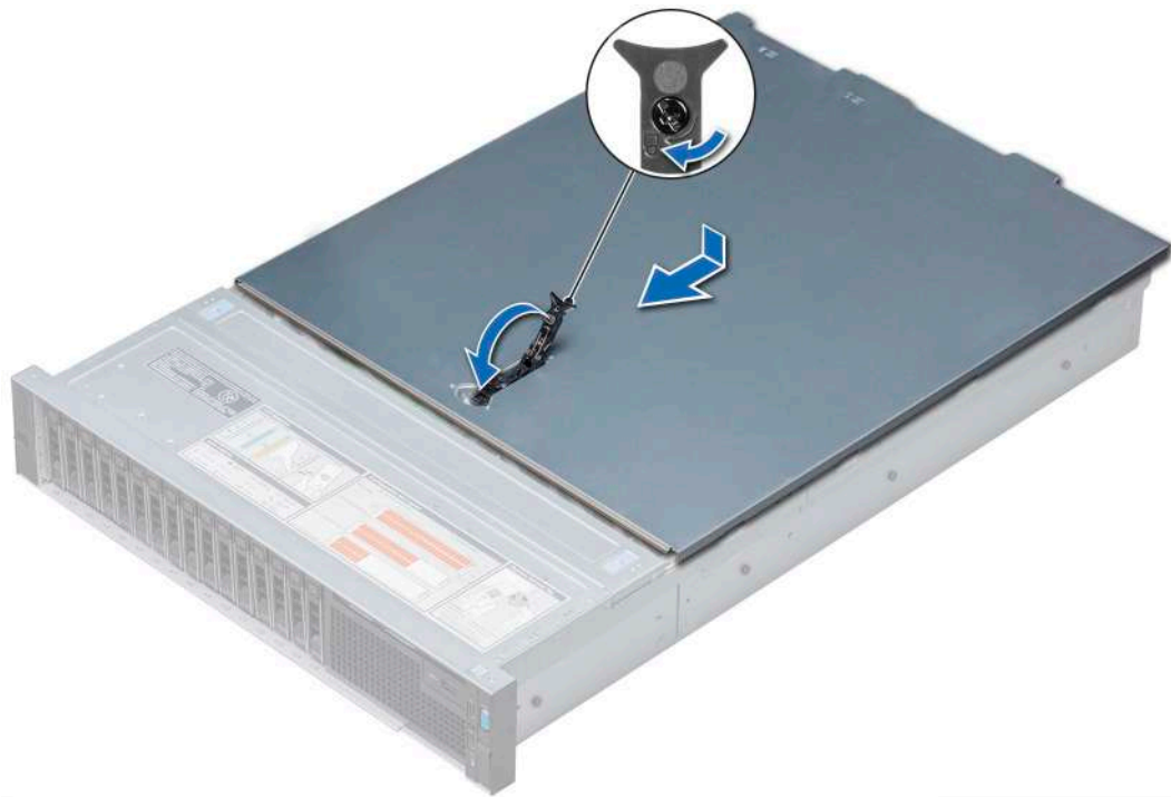
Figure 26. Installing system cover
