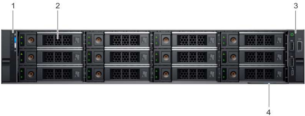
Figure 3. Front view of 12 x 3.5 inch drive system
