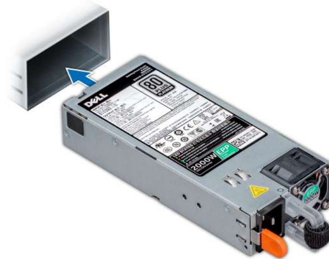
Figure 166. Installing a power supply unit
