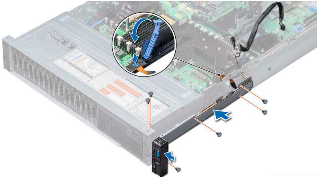
Figure 177. Installing right control panel
