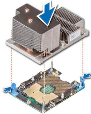
Figure 78. Installing the processor and heat sink module (2U)
