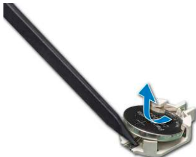
Figure 161. Removing the system battery
