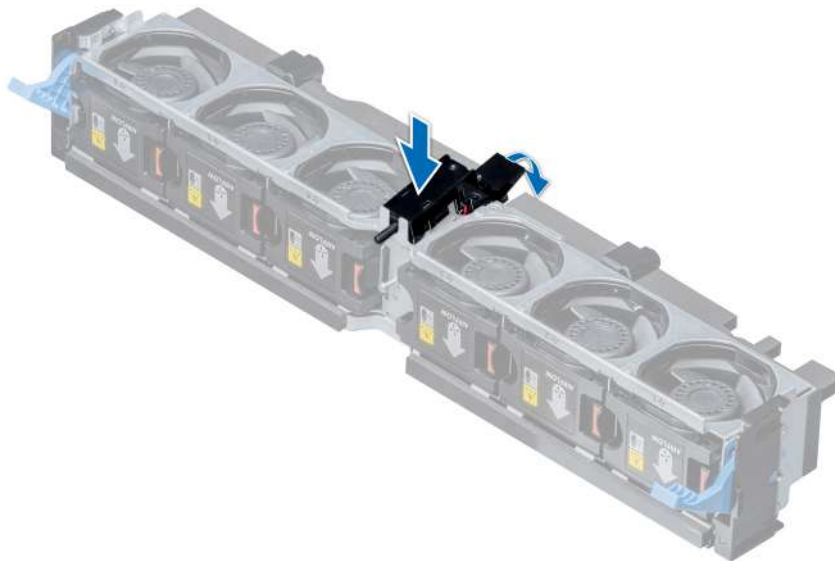
Figure 38. Installing an intrusion switch
