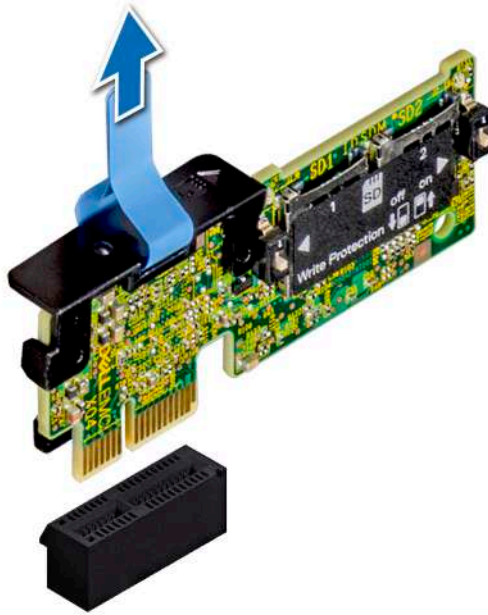
Figure 116. Removing the optional IDSDM/vFlash module
