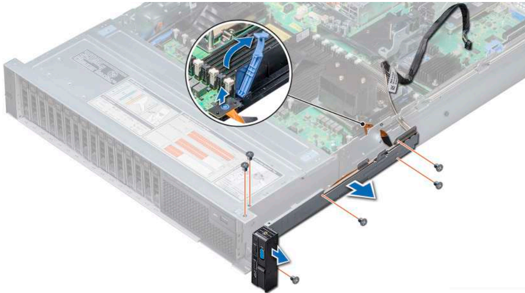
Figure 176. Removing right control panel
