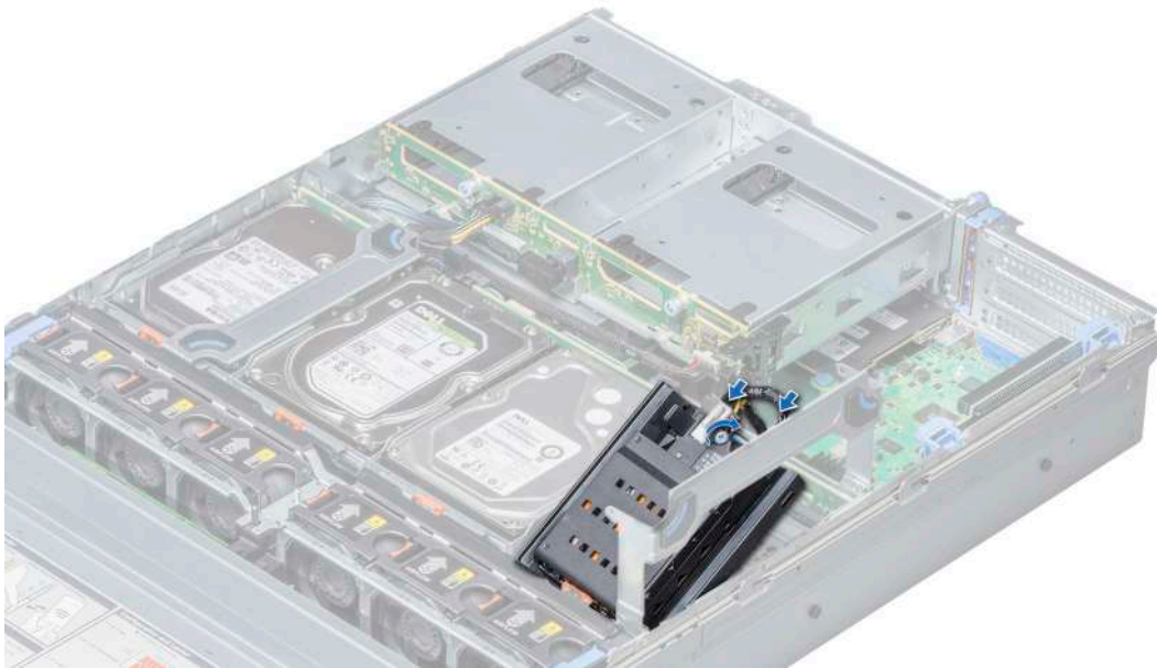
Figure 42. Installing NVDIMM-N battery into mid drive tray
