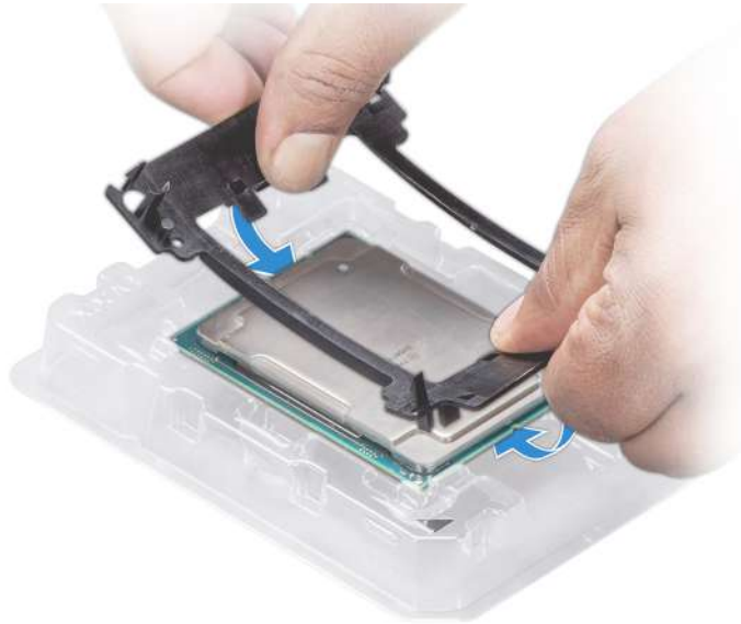
Figure 75. Installing the processor bracket
