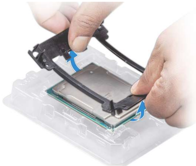
Figure 74. Removing the processor bracket
