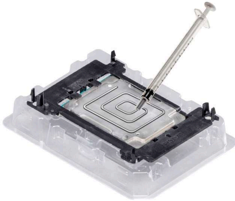
Figure 76. Applying thermal grease on top of the processor
