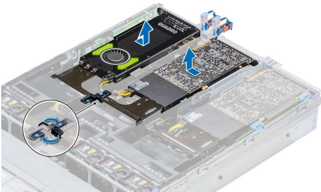
Figure 104. Removing GPU 2 and 3
