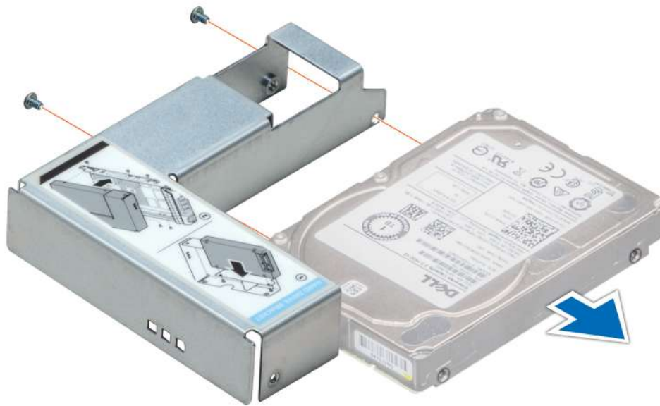
Figure 59. Removing a 2.5 inch drive from the 3.5 inch drive adapter
