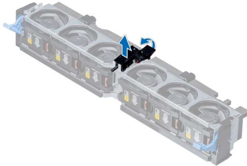
Figure 37. Removing an intrusion switch
