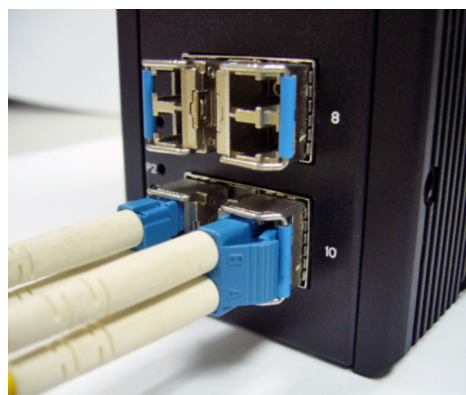
FIGURE 3-6. CONNECT THE OPTICAL FIBER TO THE SFP SOCKET
