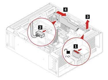
**Note:** When installing a new super capacitor module, connect the super capacitor module cable to the super capacitor module connector (J14) on the RAID card.
