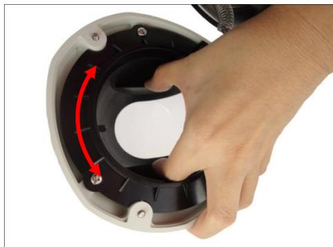
2. Tighten the three (3) screws to attach the dome cover to the camera body.
