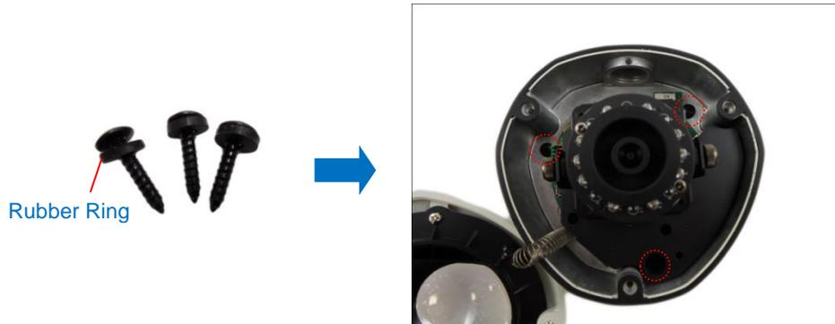
**⚠ CAUTION:** *When using electric screwdrivers*, be careful not to touch the internal camera components while attaching the screws. Since electric screwdrivers vary in sizes, speed, and force, they may bruise and damage the internal camera components.
