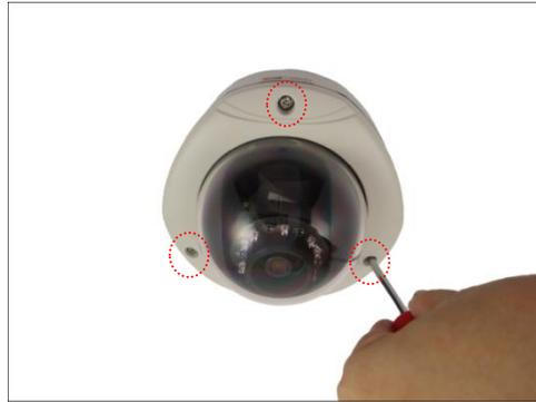
2. Using a screwdriver, remove the screw securing the spring wire to the dome cover.
