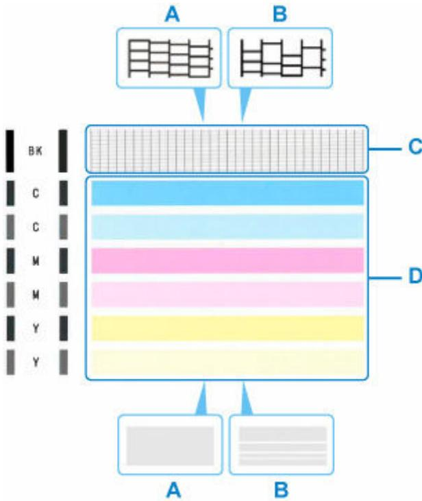
A: No missing lines/No horizontal streaks
