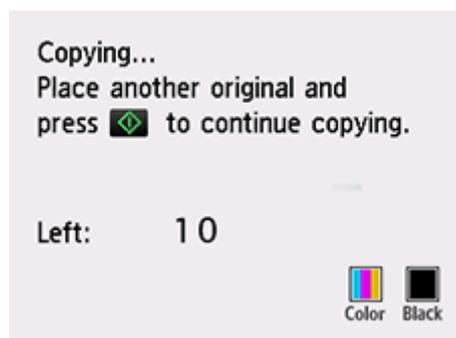
Load the original on the platen and select the same button (**Black** button or **Color** button) as the one which you previously pressed.
