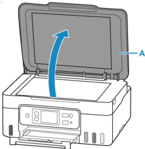
2. Load original WITH THE SIDE TO SCAN FACING DOWN on platen.
