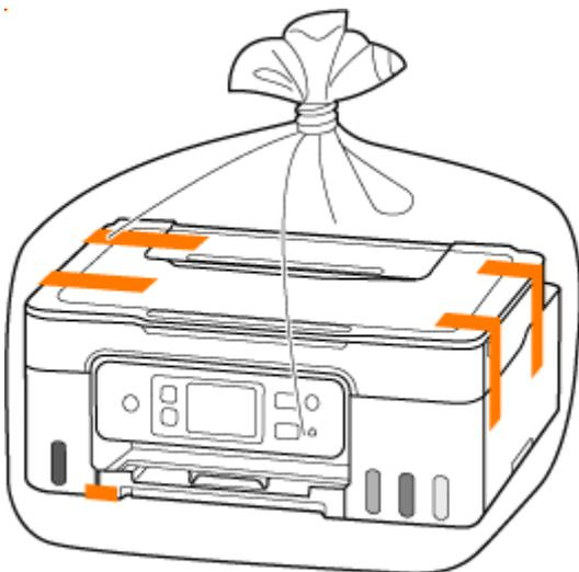
**11. Attach the protective material to the printer when packing the printer in the box.**
