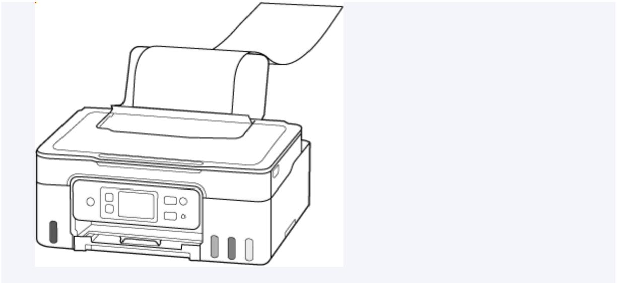
5. Move the right paper guide and adjust the guides to both edges of the paper stack.
