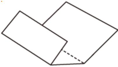
9. Load only this sheet of paper on the rear tray so that the wider folding margin is put down with the opened surface (valley fold) upward.
