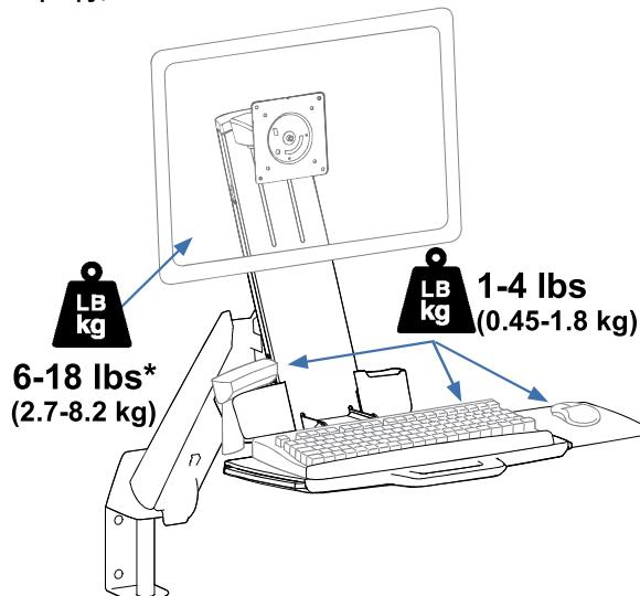
\* The Combo Arm can be modified to mount displays up to 25 lbs (11.3 kg), however display lift and tilt motion will not be possible if this option is chosen. Refer to special instructions on page 8.
