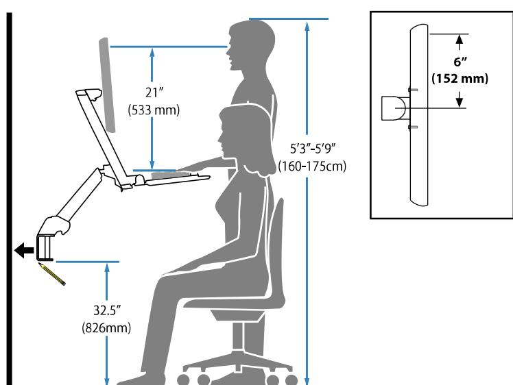
Mounting height assumes there is a 6" (152 mm) distance between the center of your monitor mounting holes and the top of the screen. If your distance is smaller, you should increase mounting height accordingly; if your distance is larger, you should decrease your mounting height accordingly.
