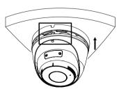
Adjust the housing to the position shown in figure above. Align the screw hole on the
