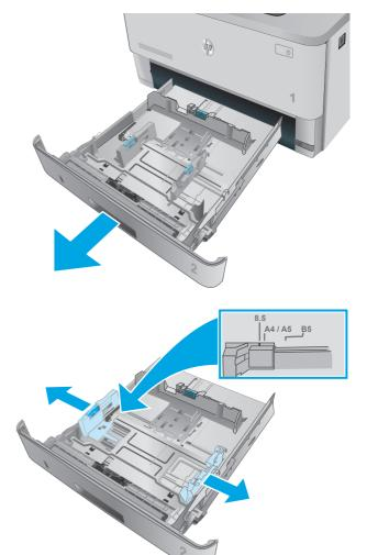
Adjust the paper-width guides by squeezing the adjustment latch on the left guide and sliding the guides to the size of the paper being used.  Adjust the paper-length guide by squeezing the adjustment latch and sliding the guides to the size of the paper being used.
