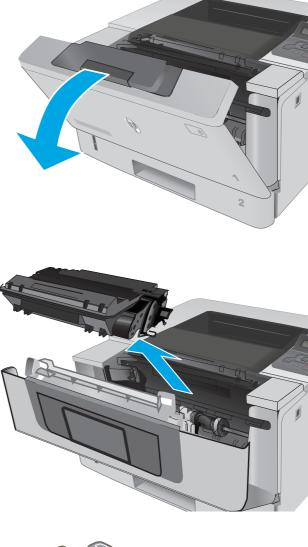
3. Remove the used toner cartridge from the printer.
