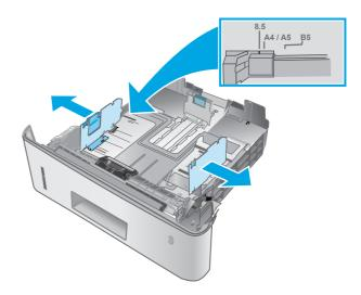
Adjust the paper-width guides by squeezing the adjustment latch on the left guide and sliding the guides to the size of the paper being used. 3. Adjust the paper-length guide by squeezing the adjustment latch and sliding the guides to the size of the paper being used.
