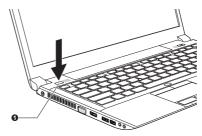
Figure 1-7 Turning on the power (R930)
