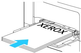
For 2-sided printing, load letterhead and pre-printed paper face down with the top edge facing you.
