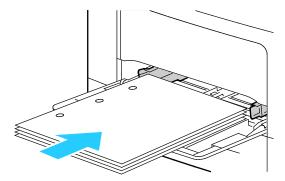
For 1-sided printing, load letterhead or pre-printed paper face up with the top edge going into the printer.
