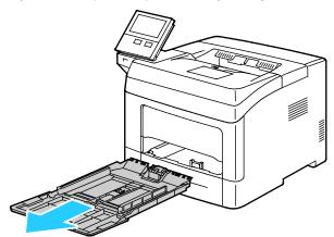
If the bypass tray is loaded with paper already, remove any paper that is a different size or type. Raise the paper stop.
