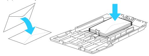
Note: Do not load paper above the maximum fill line. Overfilling the tray can cause the printer to jam.
