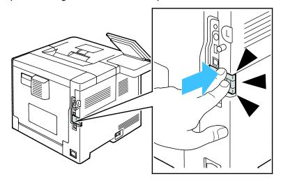
5. Place the left-side cover into position and slide it toward the front of the printer. Tighten the bolt to secure the cover.
