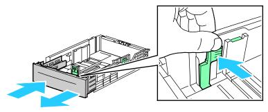
To extend the tray for longer paper, hold the back of the tray with one hand. With the other hand, press the release latch at the front of the tray, then pull the ends outward until they latch.
