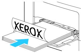
Note: Do not load paper above the maximum fill line. Overfilling the tray can cause the printer to jam.
