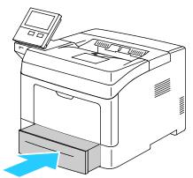
4. Load paper into the tray before inserting it back into the printer. For details, refer to Loading Paper into Trays 1–4 on page 101.
