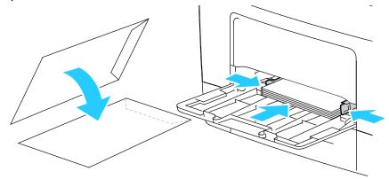
Note: For envelopes to print correctly, when you load envelopes with the flaps open, in the print driver, select **Portrait**, **Landscape**, or **Rotated Landscape**, as needed. To flip the images, in the print driver, use **Rotate Image 180 Degrees**.
