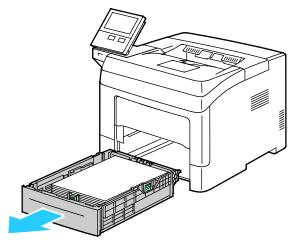
2. Adjust the paper length and width guides as shown.
