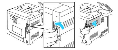
3. To remove the Wireless Network Adapter Port Cover, press the latch to the left, then pull the cover away from the printer.
