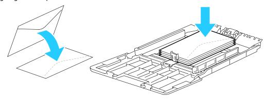
Note: When you load Monarch or DL envelopes, remove the Bypass Tray. For details, refer to Loading Small Paper Sizes in the Bypass Tray on page 107.
