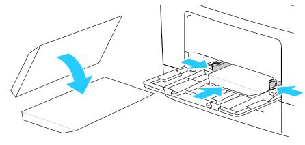
• Insert envelopes with the print side up, flaps closed and down, and flaps going into the printer.
