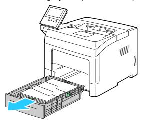
5. Remove any crumpled paper from the tray and any remaining paper jammed in the printer.
