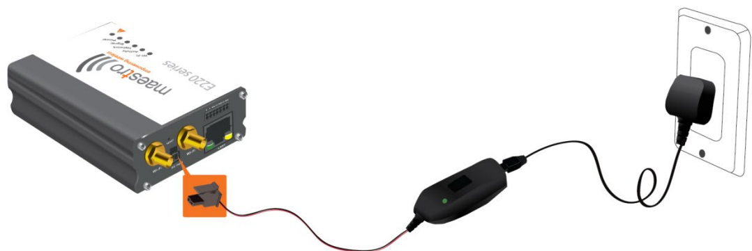
Figure 9: Connecting the AC power connector
