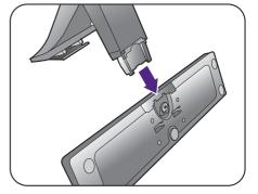
Tighten the screw on the bottom of the monitor base as illustrated.
