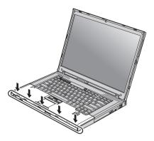
d. Close the computer display, and turn the computer over. Reinstall the four screws for the palm rest.
