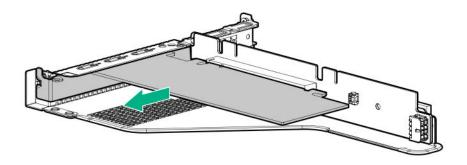
Remove the existing riser board from the riser cage.
