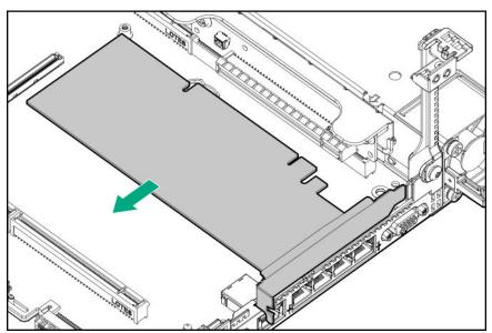
10. Remove the PCI riser cage.
