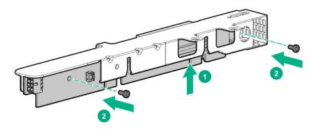
10. Install the drive cage on the riser cage.
