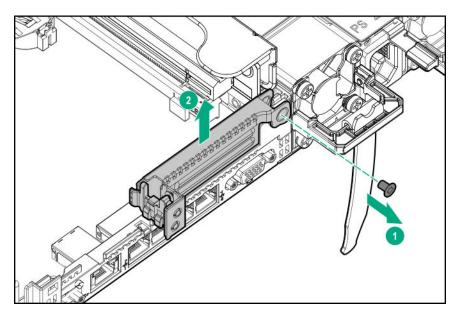
Install the full height PCIe x16 riser cage latch. Use a T-15 Torx screwdriver to remove the riser cage screw.
