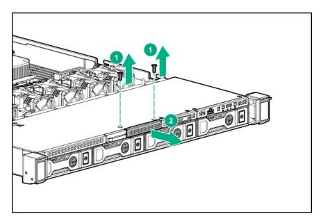
**6.** Install the 4 LFF display port/USB module.
