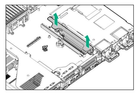
Lift and remove the secondary riser cage latch. Use a T-15 Torx screwdriver to remove the riser cage screw.
