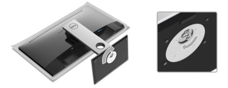
7 After fully tightening the screw, fold the screw handle flat within the recess.
