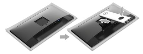
4 Hold the stand base with the triangle mark,  $\blacktriangle$ , facing upward. Then, align the stand base protruded blocks to the matching slot on the stand.
