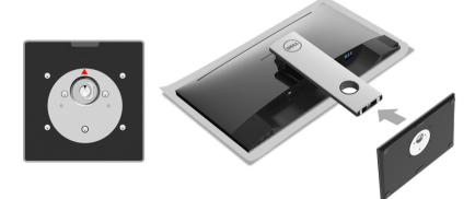
5 Insert the stand base blocks fully into the stand slot.
