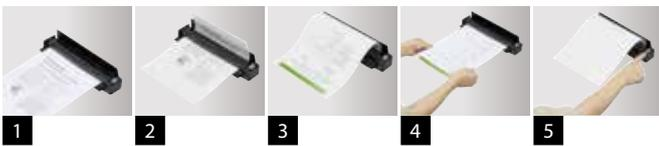
**1** Insert the page face up and press the Scan button. **2** The iX100 proceeds to scan the front side using the U-turn path. **3** The page exits facing front side down. **4** Reinsert the page without pressing the Scan button. **5** The page is scanned. Press the Scan button to end the scanning process and create the PDF image file.
