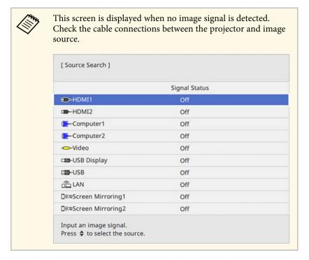
• Press the button for the source you want on the remote control. If there is more than one port for that source, press the button again to cycle through the sources.
