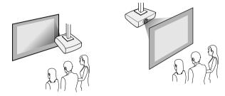
Select the correct **Projection** option in the projector's **Installation** menu according to the installation method being used. If necessary, adjust the **Menu Rotation** setting in the projector's **Display** menu.
