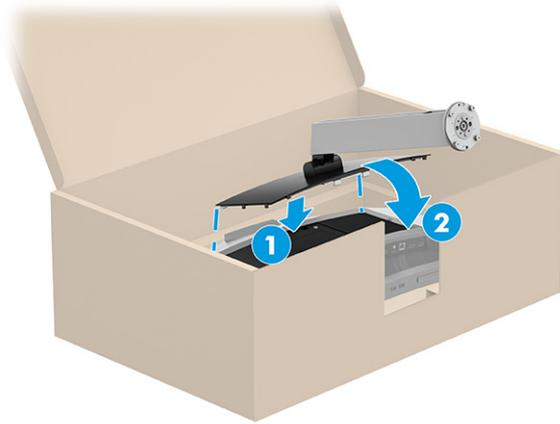
3. Place the base on the bottom the stand (1), and swivel the base counterclockwise to lock it in place (2).
