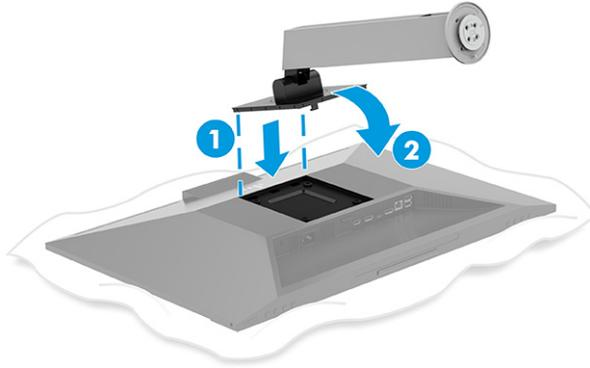
4. Place the base on the bottom the stand (1), and swivel the base counterclockwise to lock it in place (2).
