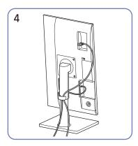
Put both cables in the cable holder on the stand (HOLDER-STAND CABLE) to organize the cables, as shown in the figure.
