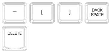
In addition to the 3Dconnexion Keys, your Numpad Pro provides five Globally Programmable Keys, whose function remains the same system-wide (no matter in which application you are currently working). They can be easily personalized in the **3Dconnexion Settings**.
