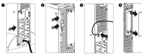
If Required, Connect the Emergency Power Off (EPO) Feature
