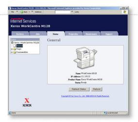
An Embedded Web Server (EWS) allows you to monitor print jobs and run status using a PC browser. Users can set print and fax functions from the PC. Network administrators can better understand and support the office's printing needs.
