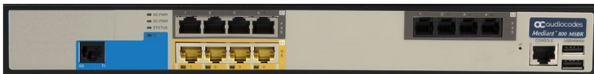
Figure 6-14: Connecting T1 WAN Port – Mediant 800C MSBR
