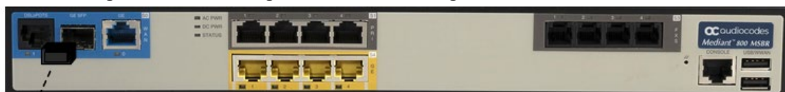
Figure 6-5: Removing Protective Dust Plug – Mediant 800C MSBR
