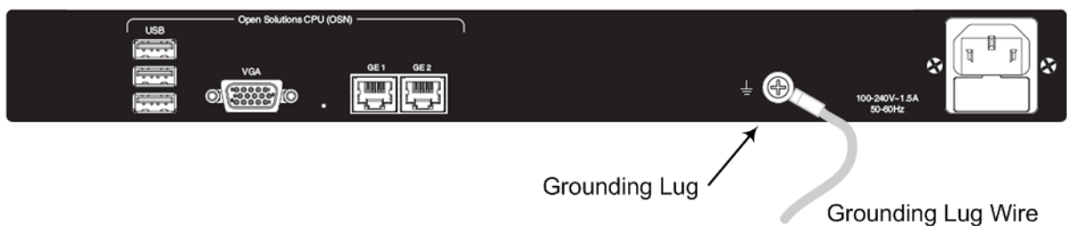
Figure 6-1: Earthing the Device
