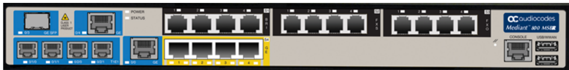
Figure 6-13: Connecting E1/T1 WAN Port – Mediant 800B MSBR
