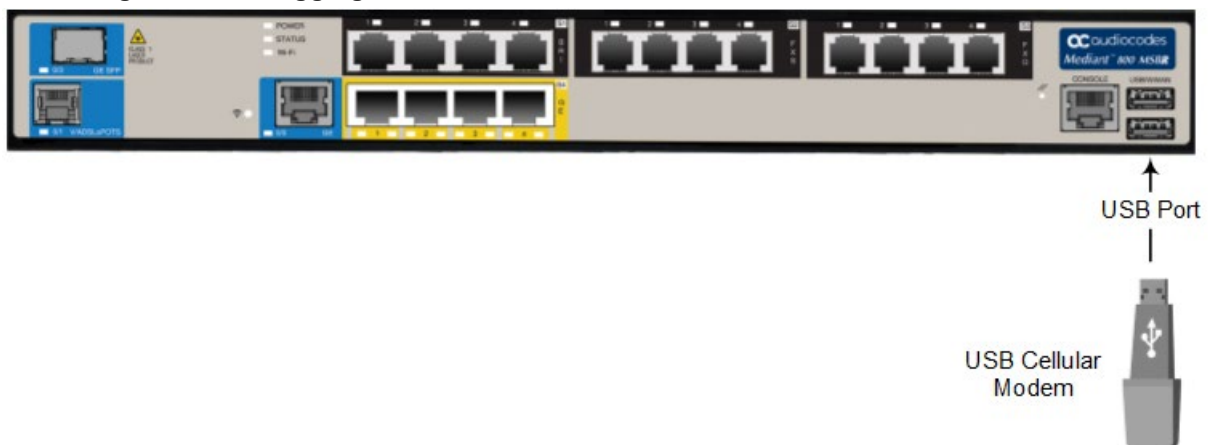
Figure 6-15: Plugging 3G/4G Cellular Modem into USB Port – Mediant 800B MSBR
