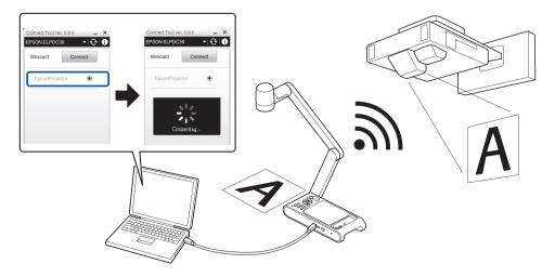
**Note:** For Epson projectors, you need to select **Screen Mirroring** as the source to connect via Miracast.
