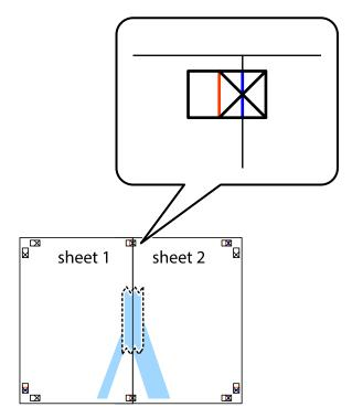
3. Cut the taped sheets in two along the vertical red line through the alignment markers (this time, the line to the left of the cross marks).
