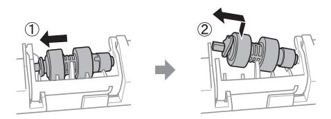
12. Insert the shaft of the new maintenance roller into the hole in the holder, and then slide the shaft on the lever side along the slot while it is facing the flat surface at the front.
