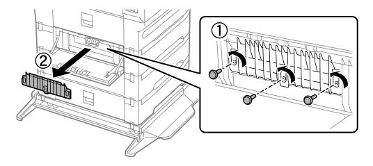
6. Slide out two used maintenance rollers, and remove both of them.
