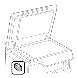
3. Use the cleaning cloth to clean the surface of the scanner glass.
