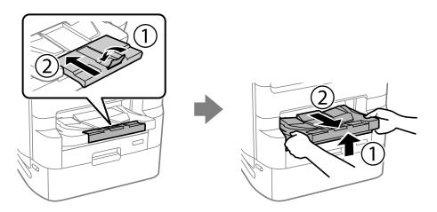
Remove the printer stand from the box, and then remove any protective materials.
